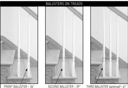
Adjustments to rake rail heights from 34" can be accommodated on a 1:1 basis. Examples: For a 36" rail height, simply add 2" to the given length and order the nearest baluster length *(rounding up if necessary)*. For a 30" rake rail height, subtract 4" from the given length and order the nearest baluster length *(rounding up if necessary)*.
