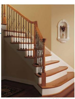
Shown: C-6210 Handrail, C-7210 Starting Easing w/ Cap, C-7214S Upeasing, C-7220 Tandem Cap, C-4011 Newel, SAT-1BASK, SAT-2BASK, SAT-FSH-01
