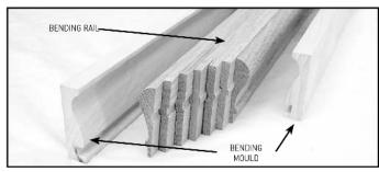
The key components of curved rail construction are bending rails and bending moulds. Bending rail is most easily understood when imagining a standard rail profile cut into thin, vertical strips. Bending mould is a form, moulded to the outside profile of the handrail, that is used to cradle the bending rail as it is being shaped to the stair.
